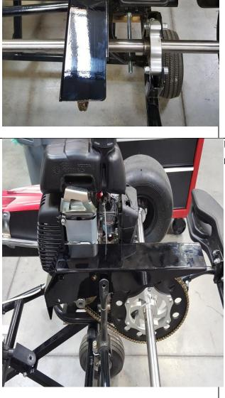
Use the three bolts supplied in the kit to mount the chain guard.
