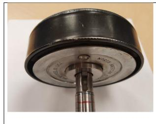
Slip the clutch unit onto the crankshaft.
