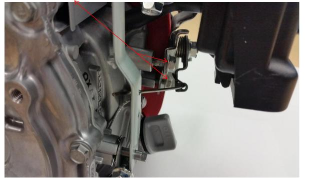
2. Before you complety tighten up the throttle bracket, make sure the "S" bend is tucked behind the throttle bracket.
