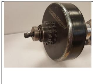
Insert the bolt into the hat spacer and torque the bolt to 14 foot-pounds.
